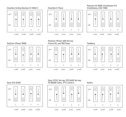
Figure 11. DIP switch configurations
